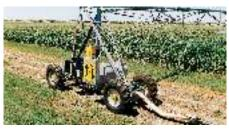
Center-feed or end-feed hose drag linear (with buried wire or above ground cable guidance)
